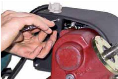
Mount the cover by using the 4 screws previously removed
