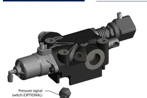
Proportional pneumatic tipping valve suitable for large oil flow applications especially designed for heavy-duty tipper bodies/semi-trailers with two different working pressures which can be selected pneumatically. Operated by proportional cab control.
