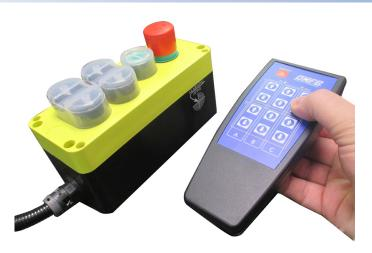
5. On the transmitter: press one of the function buttons (channel 1 Up/Down or channel 2 Up/Down) in the column on which you wish to program the receiver (A, B or C).
