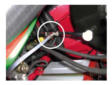
Solenoid valves suggested mounting side: engine area.
