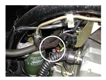
Solenoid valves suggested mounting side: on the chassis or on the frame rear the cab.
