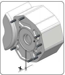
5) Keep the ring pressed into its seat and check the value between gearbox surface and ring surface ( value old X ).
