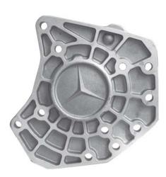
Check the rear of the gearbox to see whether it has a cover like the one illustrated in the photo, use P/N 93-16-15 for gearboxes without retarder or P/N 93-16-24 for gearboxes with retarder. Then follow the assembly instructions in 1-2-3 pages, without point 4 because there isn't the oil lube pump.
