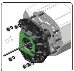
**Making sure that** both gasket and shims stay in their positions (possible use some grease), carefully mount the full assembly composed of plate, quill shaft, gasket and shims into the gearbox. To match easily the toothing of the gearbox oil pump and the groove end of the shaft help yourself with a threaded rod or M12 stud screwed into the thread of the shaft itself.
