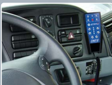
in the CABIN: Ergonomic Control Unit fixed on the dashboard or near the driver's seat.
