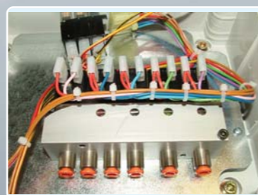
Emergency Controls: In case of failure you can manually perform the required functions.
