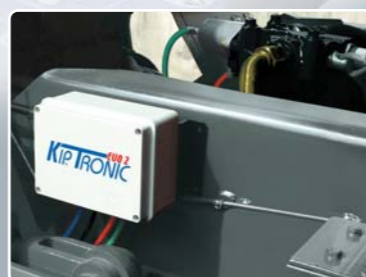
On the CHASSIS: External Box, housing the wiring, the Logic Unit and the pneumatic connections.
