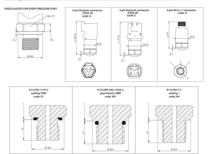
Tightening torque = 30 Nm (Max)
